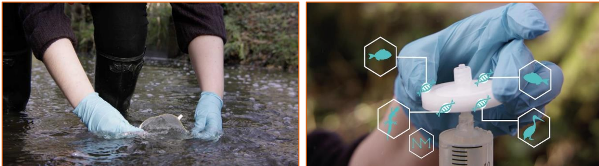
Figure 9: DNA filter unit for aquatic samples allows anyone to collect samples, democratizing biodiversity data collection. Figure from NatureMetrics 2021.
